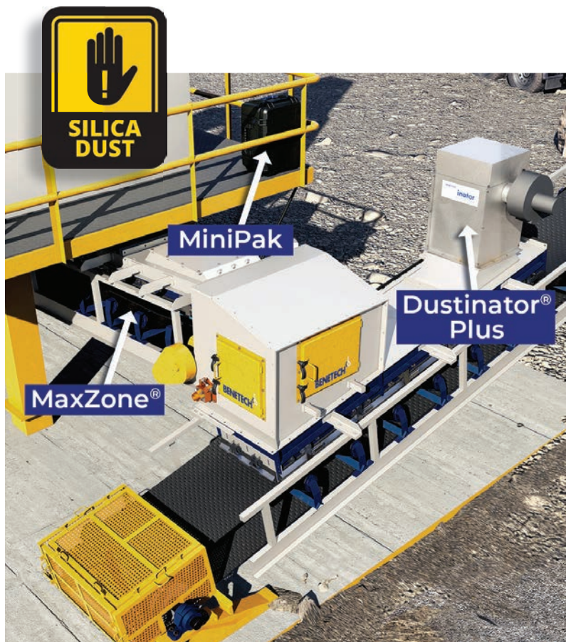
The MaxZone Safe+® is a synergistic system of bulk material containment, dry dust filtration, and fine dust agglomeration.
