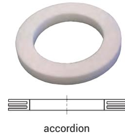
NOTE: The torque (force) required to close the handles on a pair of cam & groove fittings will vary according to the gasket chosen. Due to the nature of the PTFE material, the various PTFE gasket designs will require the most torque, increasing as you go from envelope to encapsulated, and finally, accordion.
