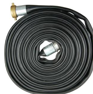
Coupled with NST (NH) female and male King short shank couplings, crimp sleeve, aluminum shank with brass pin lug swivel nut
