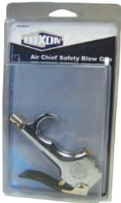
The Air Chief safety blow gun is designed to conform to OSHA Standard 1910.242 (B) permitting a maximum of 30 PSI outlet pressure when dead ended based on a maximum of 150 PSI inlet pressure, as well as OSHA Standard 1910.95 regulating occupational noise level exposure. *Safety glasses or shield must be worn when using any blow gun.*
